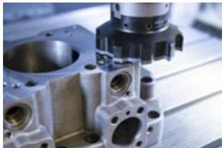
Pièce: Carter hydraulique (fonte grise) Outil: MX boronite
